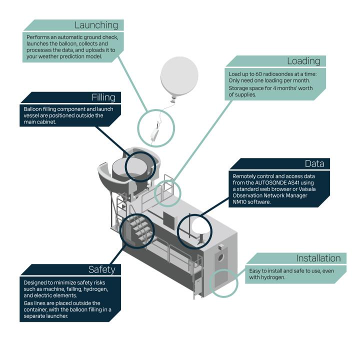
Vaisala AUTOSONDE stations have been proven in a wide range of climates through years of intensive study and testing. They are an integral part of many national upper-air networks.
